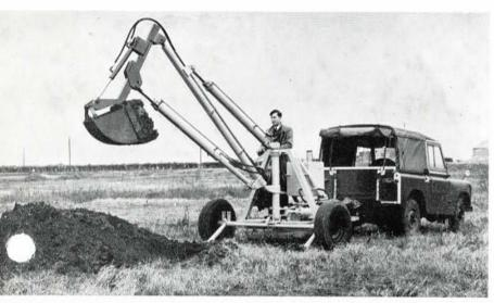
Fitted with trench hoe and tilting ram for digging a farm drainage trench. (Right) The coupling between the Land-Rover and A.T.O.S., showing the Atkinson flexible guard for the propellor shaft.
