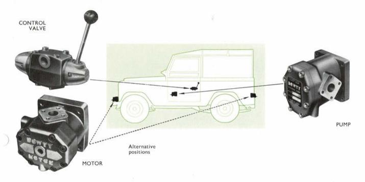
Priven by a centre p.t.o. shaft the Dowty GP.2/65 gear pump as fitted to the Land-Rover provides a simple low-cost source of hydraulic power which can be used for a variety of purposes.
