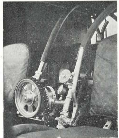
Pump and plumbing assembly in use with a 40 gallon drum.
