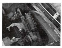
The rear p.t-o model (top) can be carried on the vehicle and is easily fitted, ready for work in under 60-seconds. The centre p.t-o model (left, shown with centre floor board removed) is also easily fitted and it may be left in position ready for immediate use.
