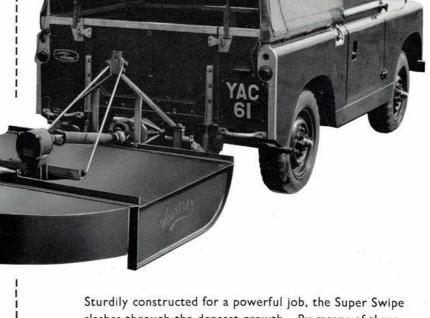
Sturdily constructed for a powerful job, the Super Swipe slashes through the densest growth. By means of three high speed revolving chains, it cuts and mulches all kinds of stalks. Its pulverising action destroys all forms of weed growth, scrub, brambles, bracken, nettles, thistles, heather, rushes, etc. Acres of land can be quickly cleared and reclaimed for cultivation—and the initial cost is extremely low.
