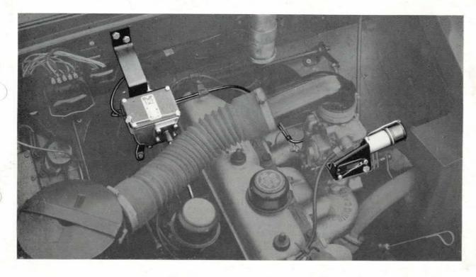
This system of vehicle road-speed limitation is offered in kit form comprising a centrifugal switch, a throttle control unit, all parts required for fitting to the particular vehicle concerned, and all necessary fitting instructions.
