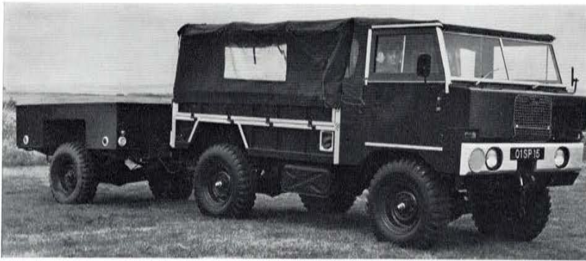
(Left) A military version of the now obsolete Land-Rover Forward Control vehicle with a powered-axle trailer.
