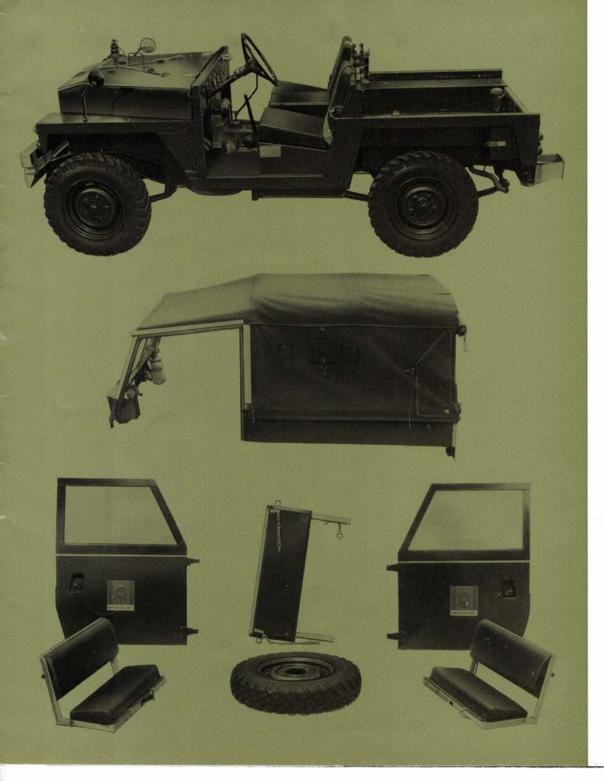
When necessary, the half-ton can be more easily reduced in weight and bulk than existing Land-Rovers already in service. This is a particularly useful feature for operations involving transportation by aircraft or helicopter or for other operations on light equipment scales.
