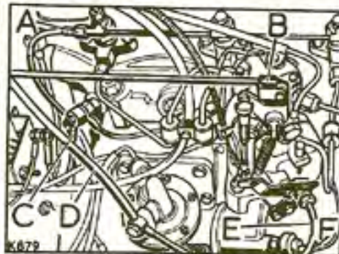
Fig. A2-16. View of engine, RH side A—Fixing for spill pipe return B—Disconnect accelerator linkage at clip C—Electrical feed to heater plugs D—Fuel pipe to fuel pump E—Fuel return pipe F—Oil pressure switch lead
