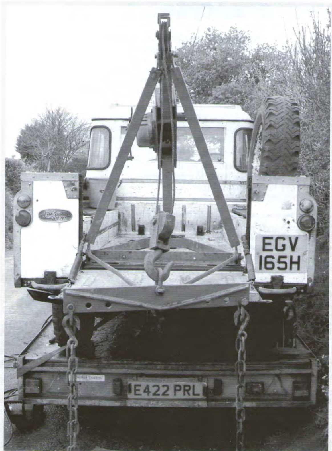
The Crane: Unknown make, does anyone know the maker? I've located several identical cranes, the winch has TFL on it but as yet we don't know who made these, they certainly don't look like the 'usual' Harvey Frost cranes as it uses a square steel stock frame, rather than round.
