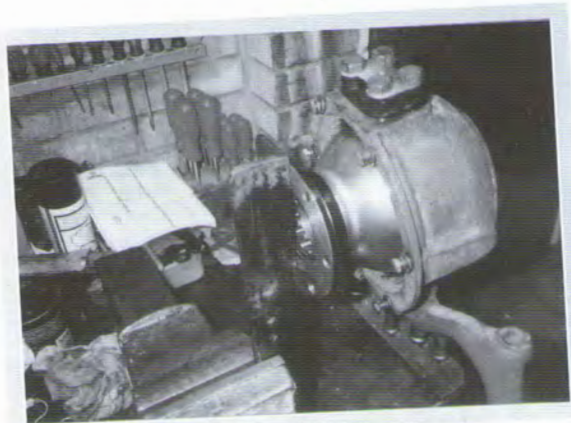
6. This is another view of the hub, I always clean out/ tap out (if necessary), any screwed holes so that all the screws fit without any problems.
