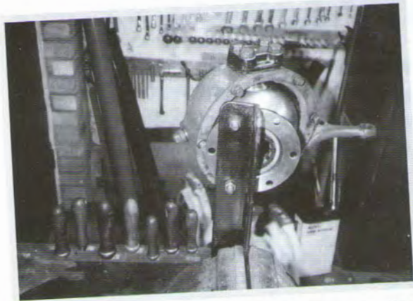
2. Another view showing how the chrome ball is mounted in holes "off centre"
