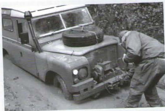
LWB IIA off roading near the river – self extraction with a winch
