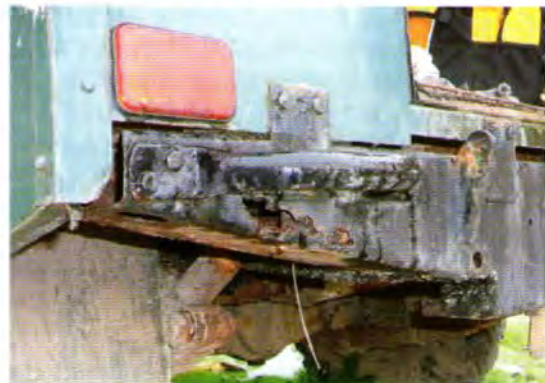
More shots showing the various forms that rot can take within the chassis and bulkhead (above and left).
