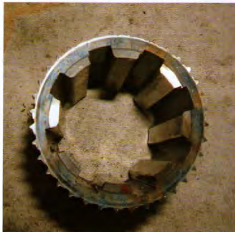
Figure 1 – Damaged Clutch sleeve
