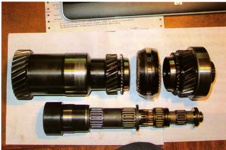
The overdrive assembly (above) and the broken bronze bush (below).
