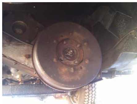
Above: Figure 1 – Handbrake assembly with drum securing nuts removed. Output flange securing nut – centre.
