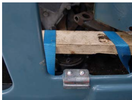
Below: Top hole blocked with a piece of wood to stop the shaft being pushed upwards. Right: Compressing the spring with a floor jack and scrap aluminium.
