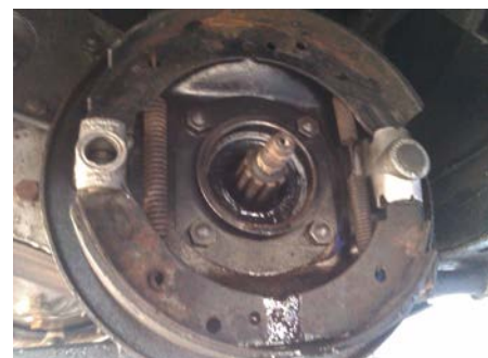
Above: Figure 3 – Oil seal with brake drum and output flange removed.
