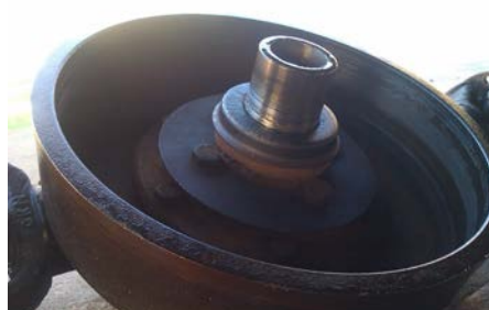
Above: Figure 2 – Drum and output flange as one assembly.
