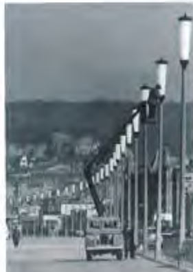
Land-Rover with hydraulic platform, this fits over the back of Mersey Tunnel - and is on the stand.
