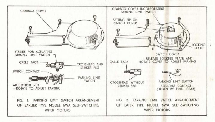
Two methods of achieving self switching have been employed with 6WA motors. In each case the necessary components - which are entirely different - are illustrated in fig. 1 and fig. 2.
