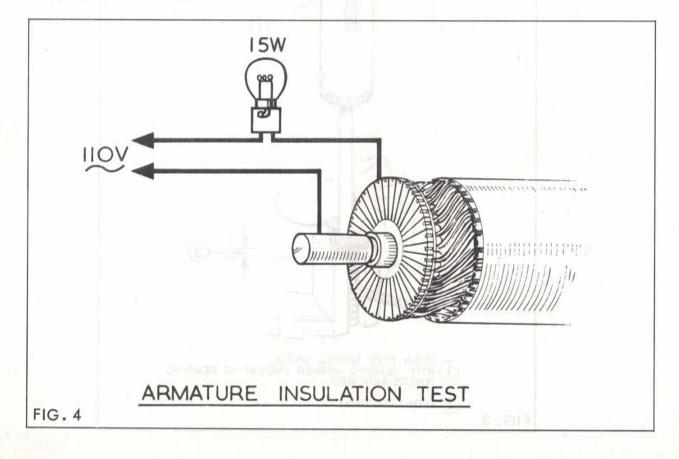
If it does the insulation has broken down, and the armature must be replaced.
