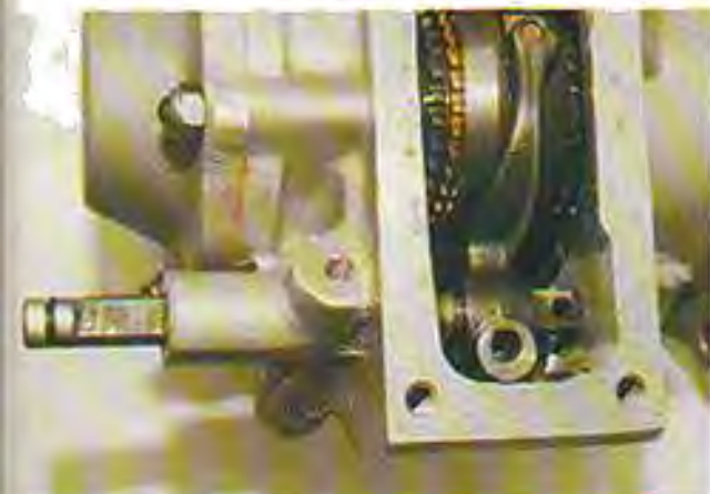
After removing the top and rear casing covers, the selector shaft is withdrawn from the casing. To do this you have to undo a pinch bolt and the selector detents
