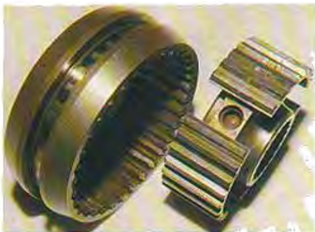
The synchroneshub hubs must be inspected for wear and damage to the teeth. Be careful not to lose the springs, chrome ball bearings and sliding blocks when dismantling
