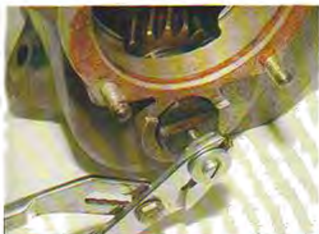
A small metric bolt is screwed into the end of the layshaft so that it can be pulled out with the aid of a wrench. This is necessary before the output gearshaft can be removed
