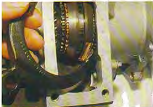
Once the selector shaft has been withdrawn, the selector fork can be lifted through the top of the casing. Note the brass swivel pads on the inner face of each fork end
