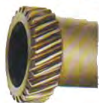
Top, position of selector fork with overdrive disengaged (left) and engaged. Above, output gearshaft teeth should look like this
