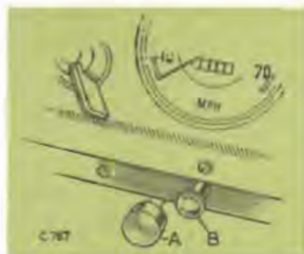
Fig. 5. Starter switch and mixture control. A—Starter switch B—Mixture control
