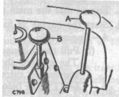
Transfer gear change lever, and front wheel drive control A—Transfer gear change lever B—Front wheel drive control
