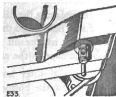
Drain tap, radiator
