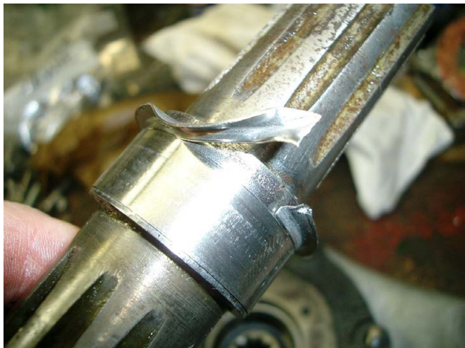
Above: Picture showing installed sleeve on a rear PTO shaft with the mounting-flange being cut and half way removed from machined groove
