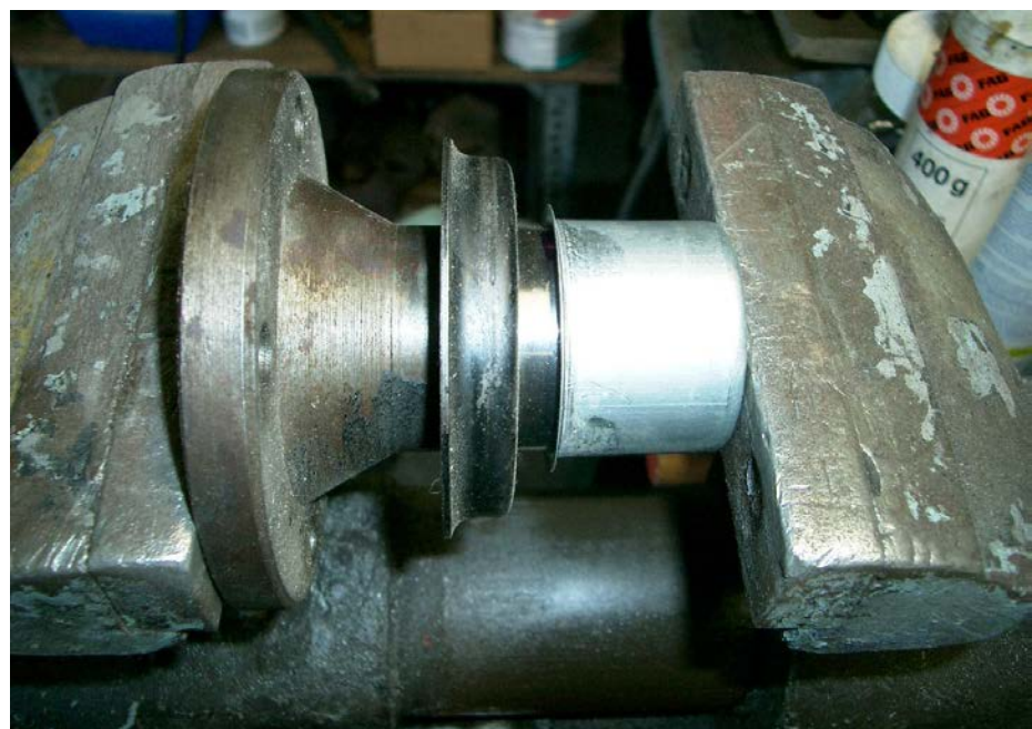
Above: Speedi-Sleeve being installed with supplied tool (far right) onto a drive flange in a vice
