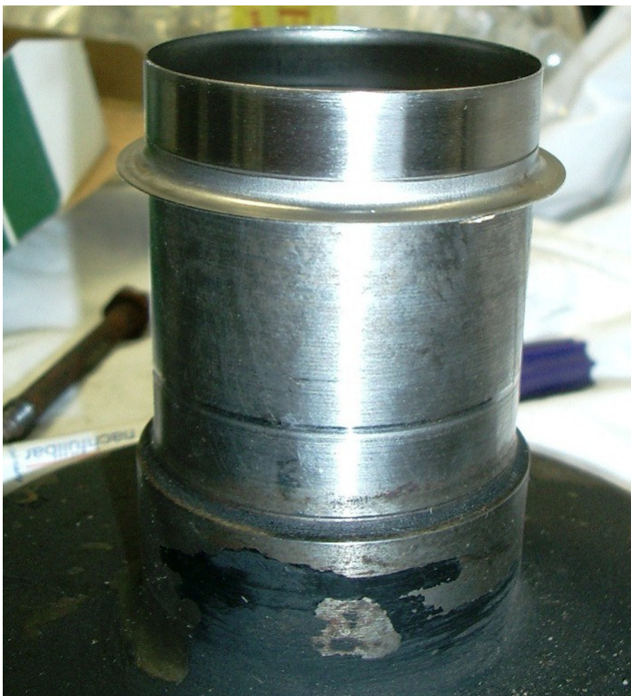
Above: SKF shaft repair sleeve positioned on top of pulley shaft
