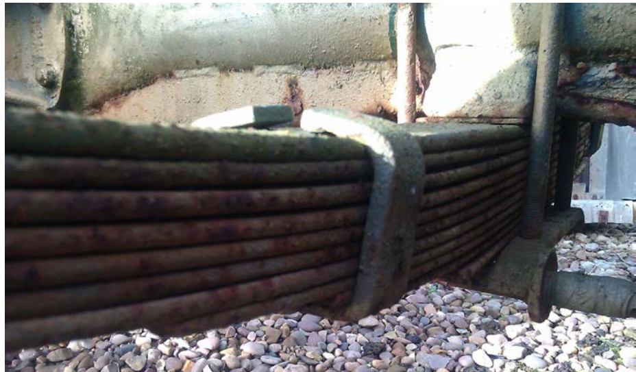
Above: A lightly corroded, probably saveable spring
