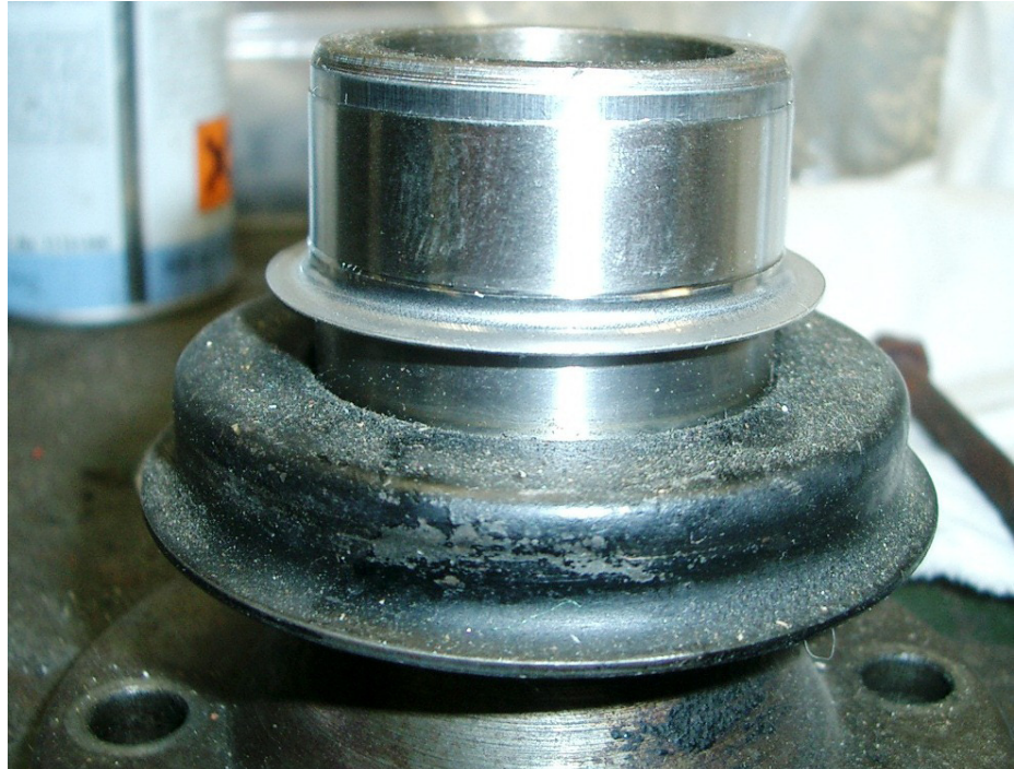
Above: SKF Speedi-Sleeve in position on a Land Rover Series 2 drive flange
