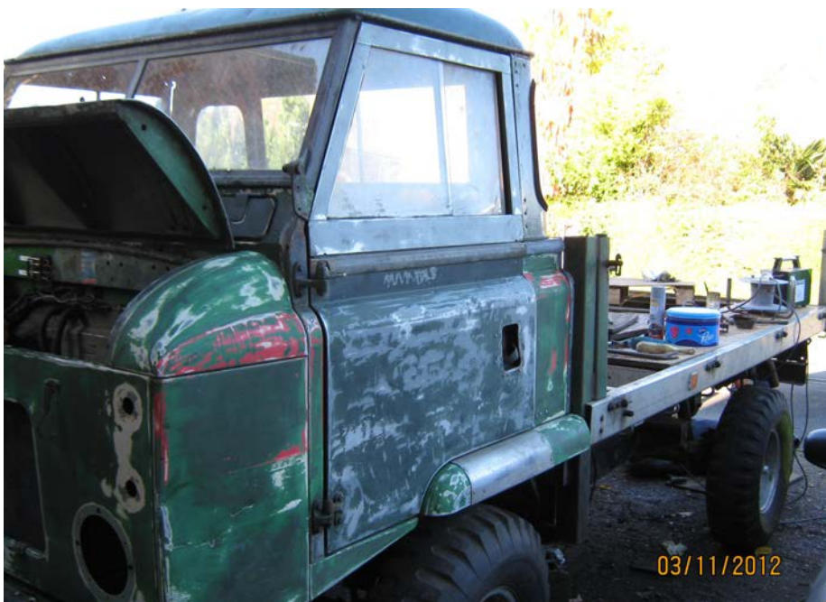
Above: Work progressing and rubbed down ready for paint...
