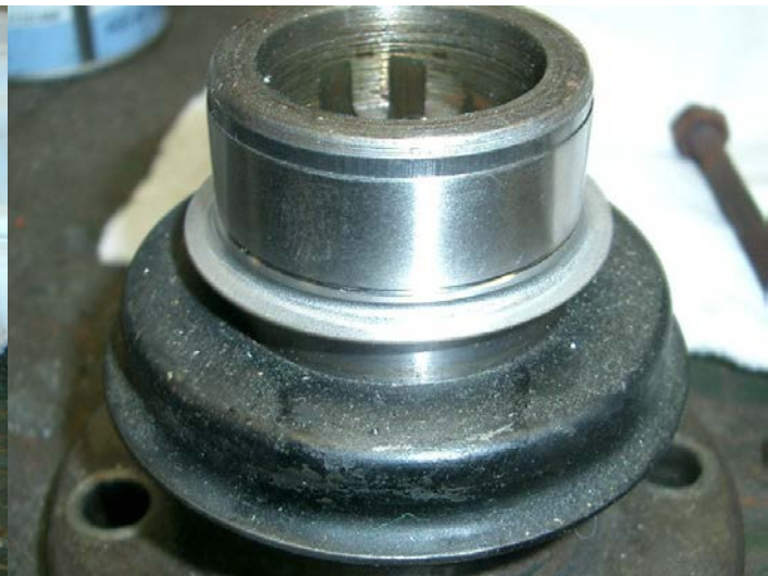
Above: Properly installed sleeve on a drive flange – mounting-flange left in position
