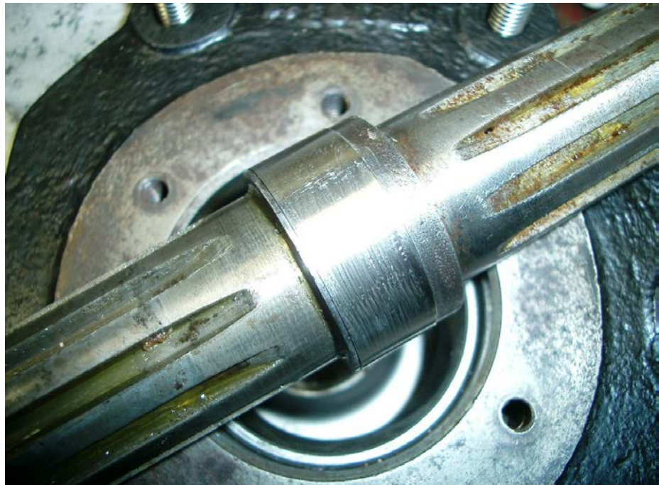
Above: Picture showing removed mounting-flange, leaving plain SKF Speed-Sleeve on PTO shaft
