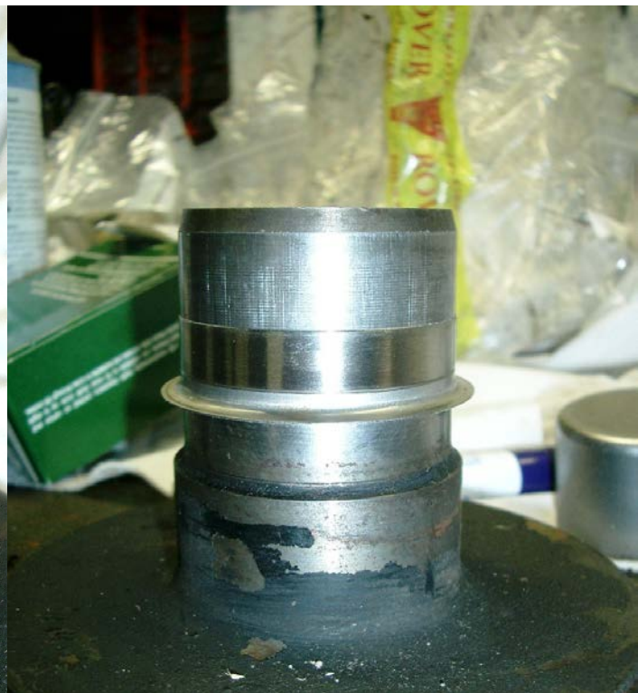
Above: Halfway down – installed with supplied tool, now just needs some more movement with the aid of a piece of tubing
