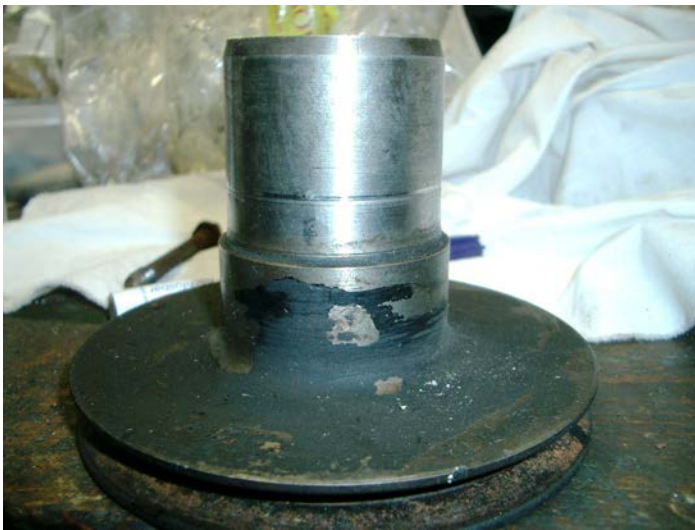
Above: Series 2 petrol engine pulley - you can see the ridge caused by the oil seal running on the same position over several decades
