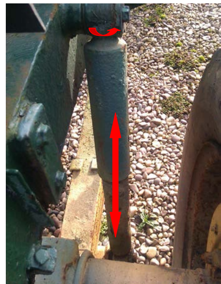
Above: Testing for wear in damper bushes
