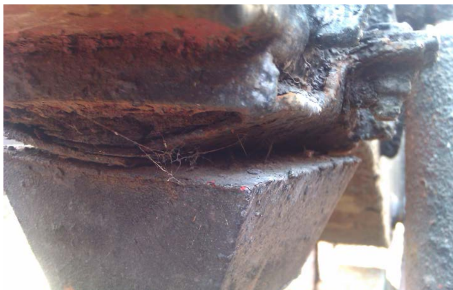
Above: Corroded bump stop mount
