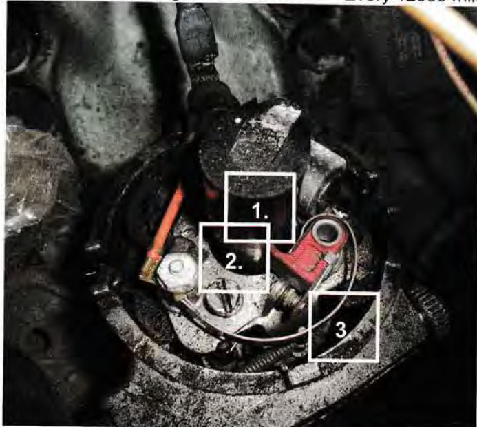
1. Lubricate cam with engine oil
