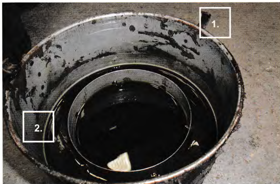
Air filter oil pan. 1. Secured to the filter by three spring clips 2. Level marked by a pressing in the side (also marked MAX) Filter oil should be the same as the engine oil
