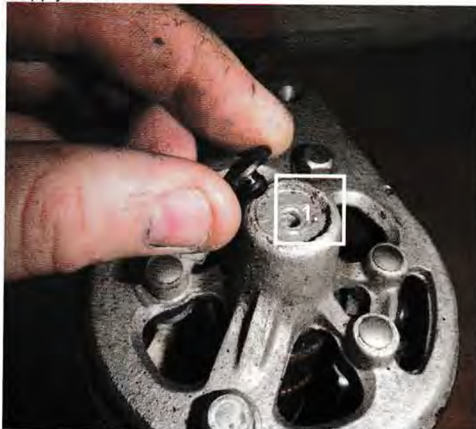
1. Remove oil way cover and apply a small amount of oil, sufficient to wet the rear bush
