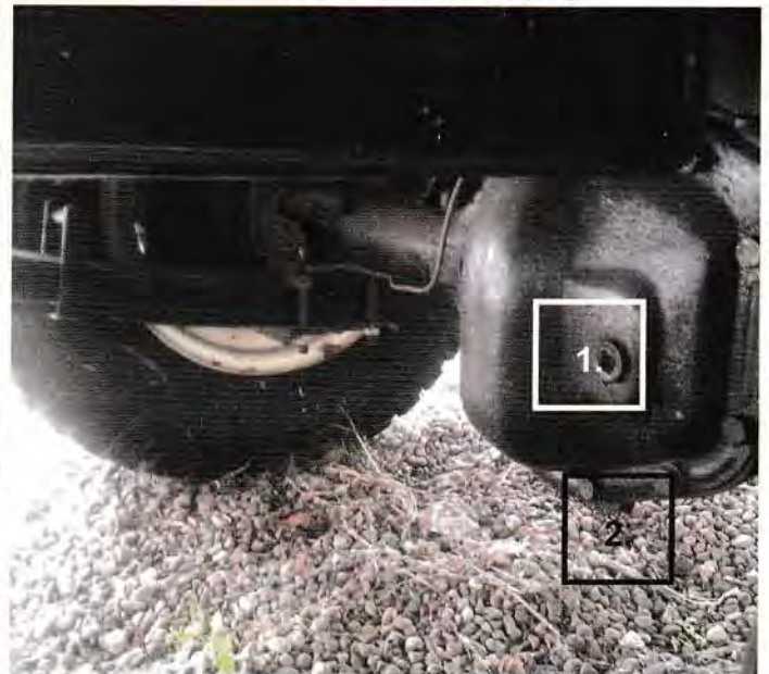
1. Salisbury diff filler/level plug 2. Rear differential drain plug
