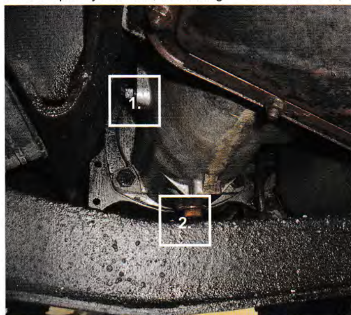
1. Gearbox level/filler plug 2. Gearbox drain plug
