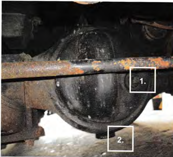
1. Front diff level/filler plug 2. Front diff drain plug
