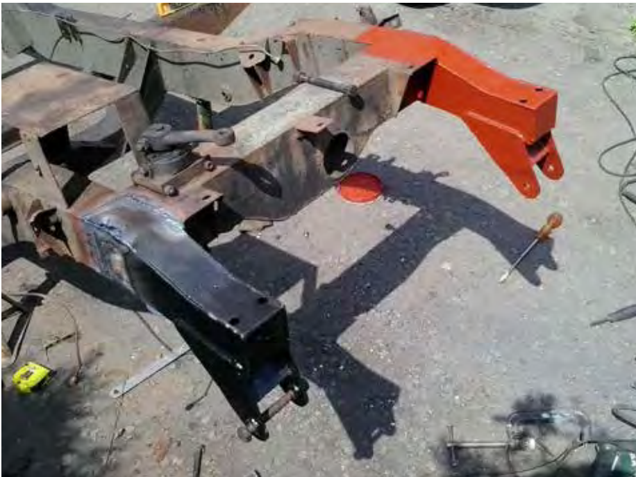
Both irons replaced: now paint, reassemble and enjoy...
