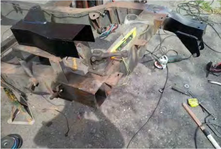
Dumb Iron cut out, note the spirit level - the chassis welder's friend...
