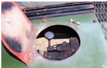
Rear PTO lever accessed by panel beneath the centre seat
