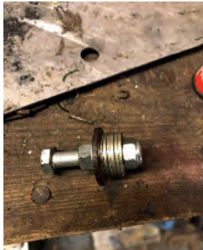
Home made tool to insert new bush
