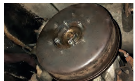
Propshafts removed to allow 'box to slide
