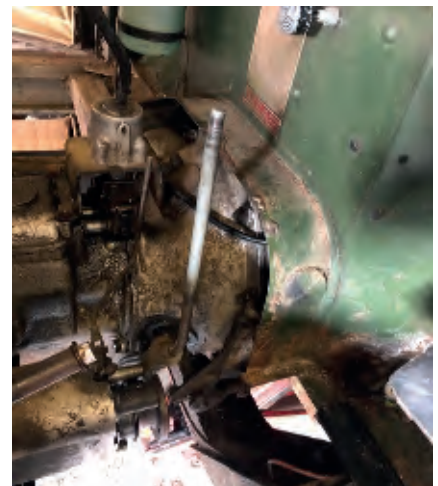
Gearbox slid back into position and secured
