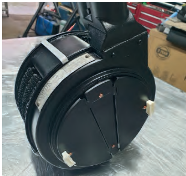
Dismantling the heater into its component parts enabled each to be tested, refurbished and the casing repainted before being put back together.
