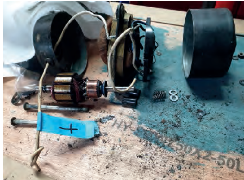
Dismantling the heater into its component parts enabled each to be tested, refurbished and the casing repainted before being put back together.
